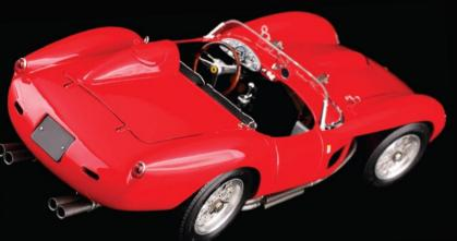
the pedal box, CMC has left nothing to chance. The exhaust system exits the front of the car via the front wings, runs under the cockpit and exits through the rear via four megaphone trumpets.
